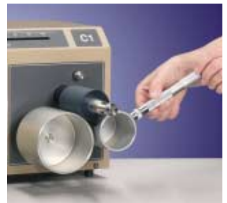
Applying ink with the IGT ink pipette
